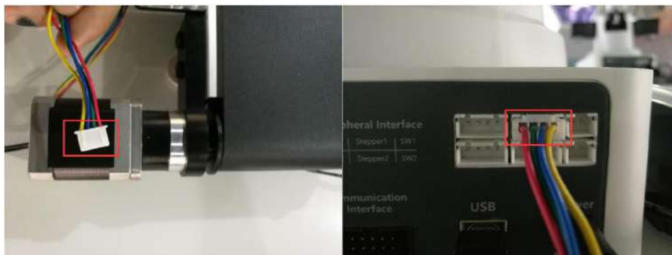
Figure 2.2 Conveyor Belt connection
