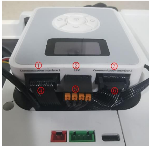
Figure 3.2 Magic Box top wiring
