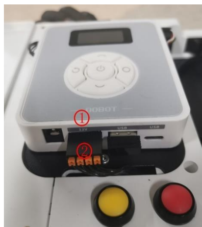
Figure 3.3 Magic box bottom wiring
