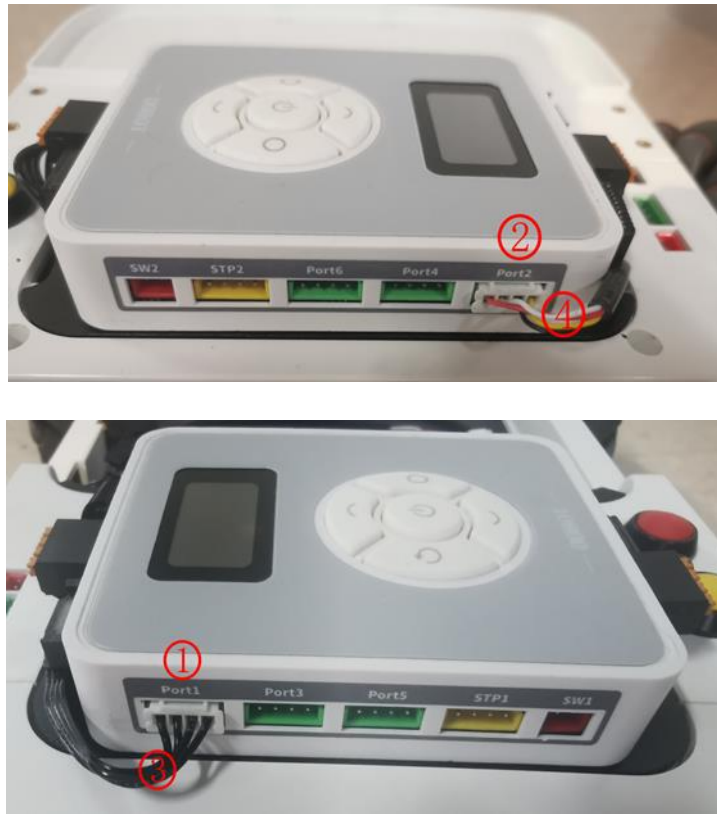
Figure 3.4 Magic Box side wiring
