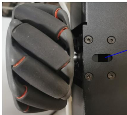
Figure 2.10 Position of motor shaft fixed screw
