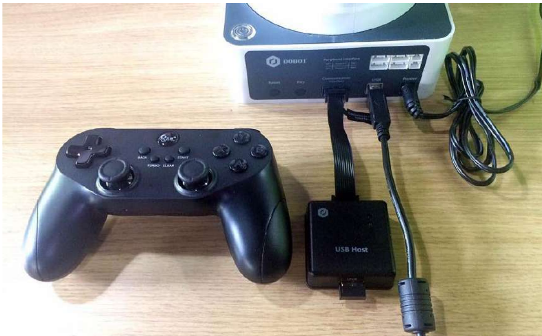
Figure 12.5 Installation of Beitong Joystick
