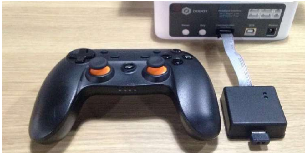
Figure 12.1 Installation of stick module
