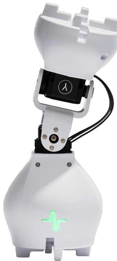
Figure 3 - Front side of a Joint Module.
