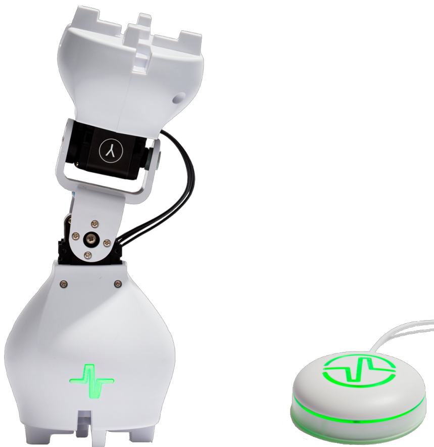
Figure 11 - Paired Joint Module with a Fable Hub.
