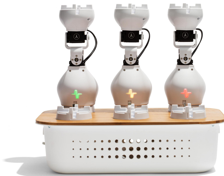
Figure 10 - Joint Modules being charged by using a charging station.
